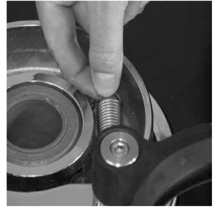
9 Once spring is removed replace Deckplate Plug and attach Pressure Arm Spring to retaining pin.
