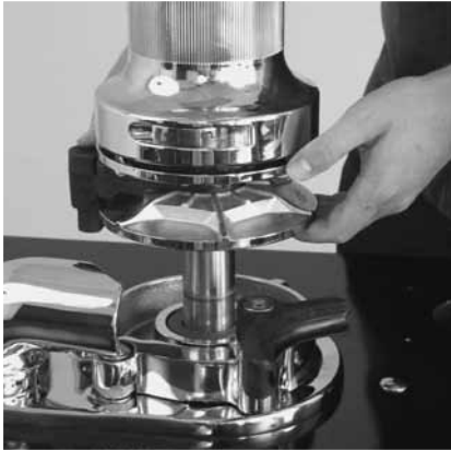
10 Apply grease to Shaft and bore, then slide into position.
