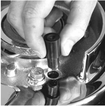
7 Temporarily remove the Deckplate Plug.
