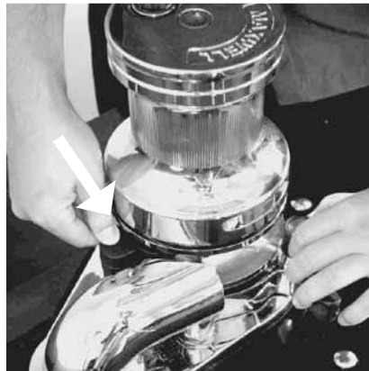
11 Make sure you align the Stripper to its locating hole (see arrow). The Pressure Arm has to be pulled away to allow easy assembly.
