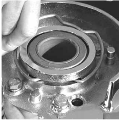
8 Remove Quick Fit Spring.
