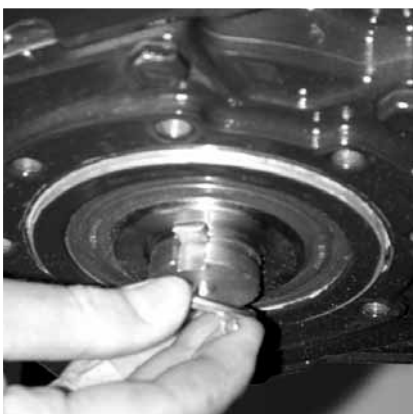
13 Finally fit the Quick Change Clip or circlip into the groove in the bottom of the Shaft.
